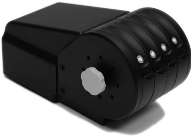
**Figure 1.** The figure represents the Cortical Metrics tactile stimulator used.
